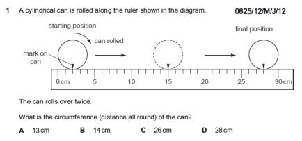
In this case, the object is 2cm ahead of the zero mark, so from the final position of the arrow deduct 2cm. Hence the final reading is 28-2=26cm. Also the cylinder is rolled twice so it covered
